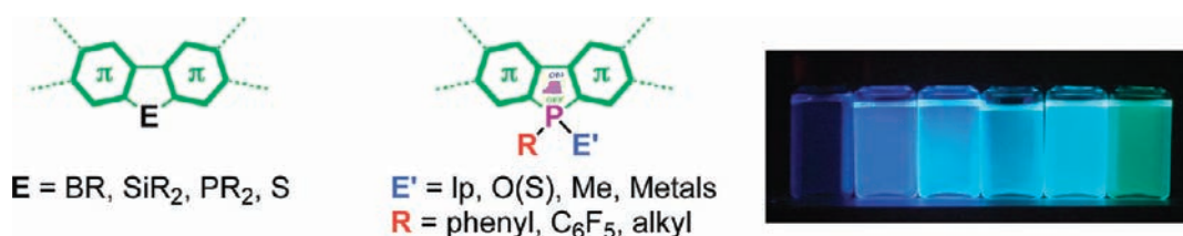
Chart 1. Heteroatom-Doped \pi -Conjugated Systems (Left) and Emission of Phosphorus-Based Conjugated Systems Based on the Nature of E' (Right)
